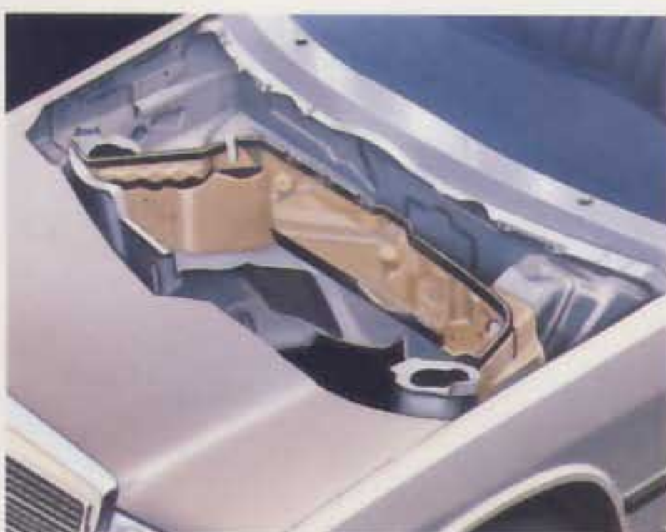
Second insulating firewall
