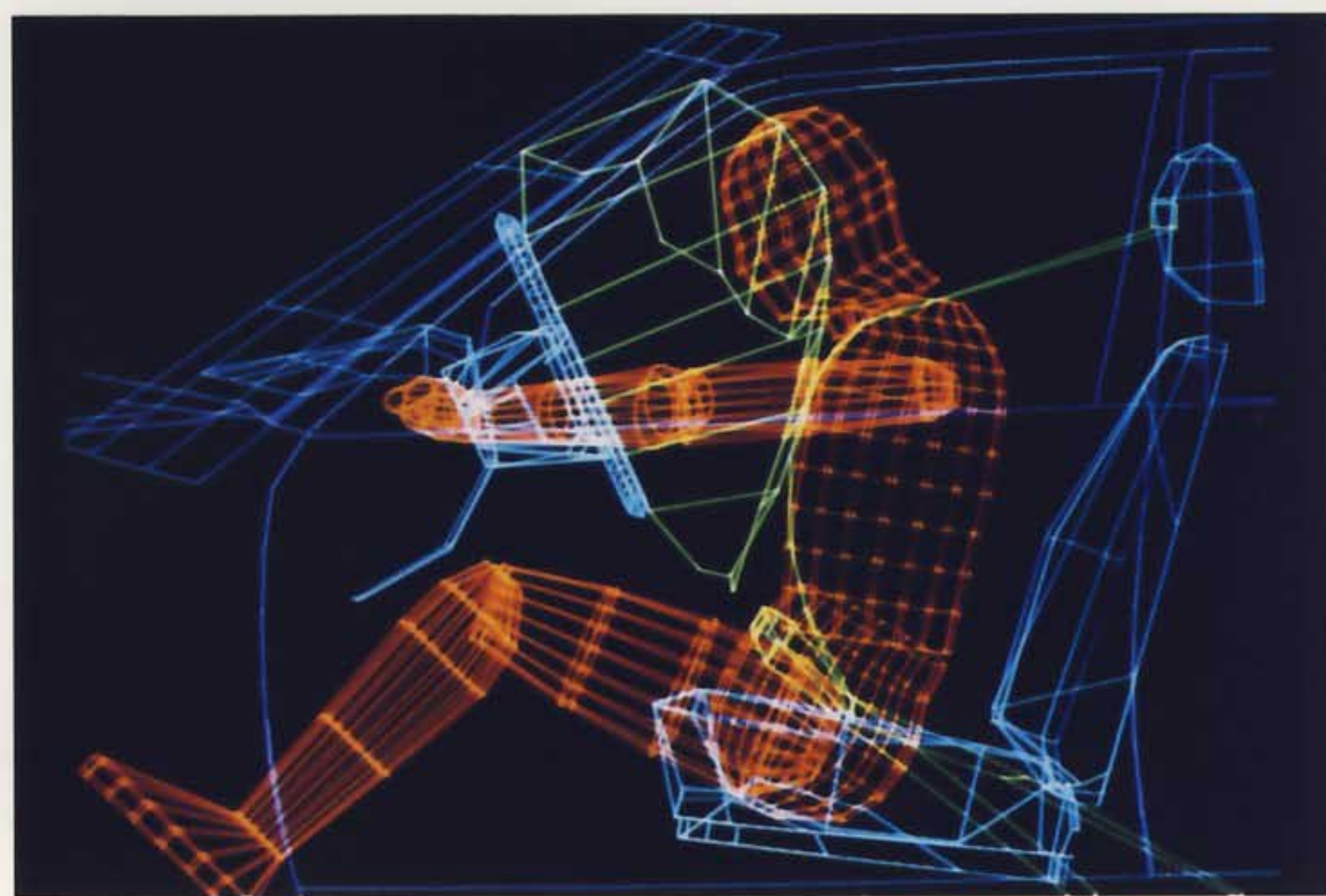
The inflated air bag in its fully extended position
