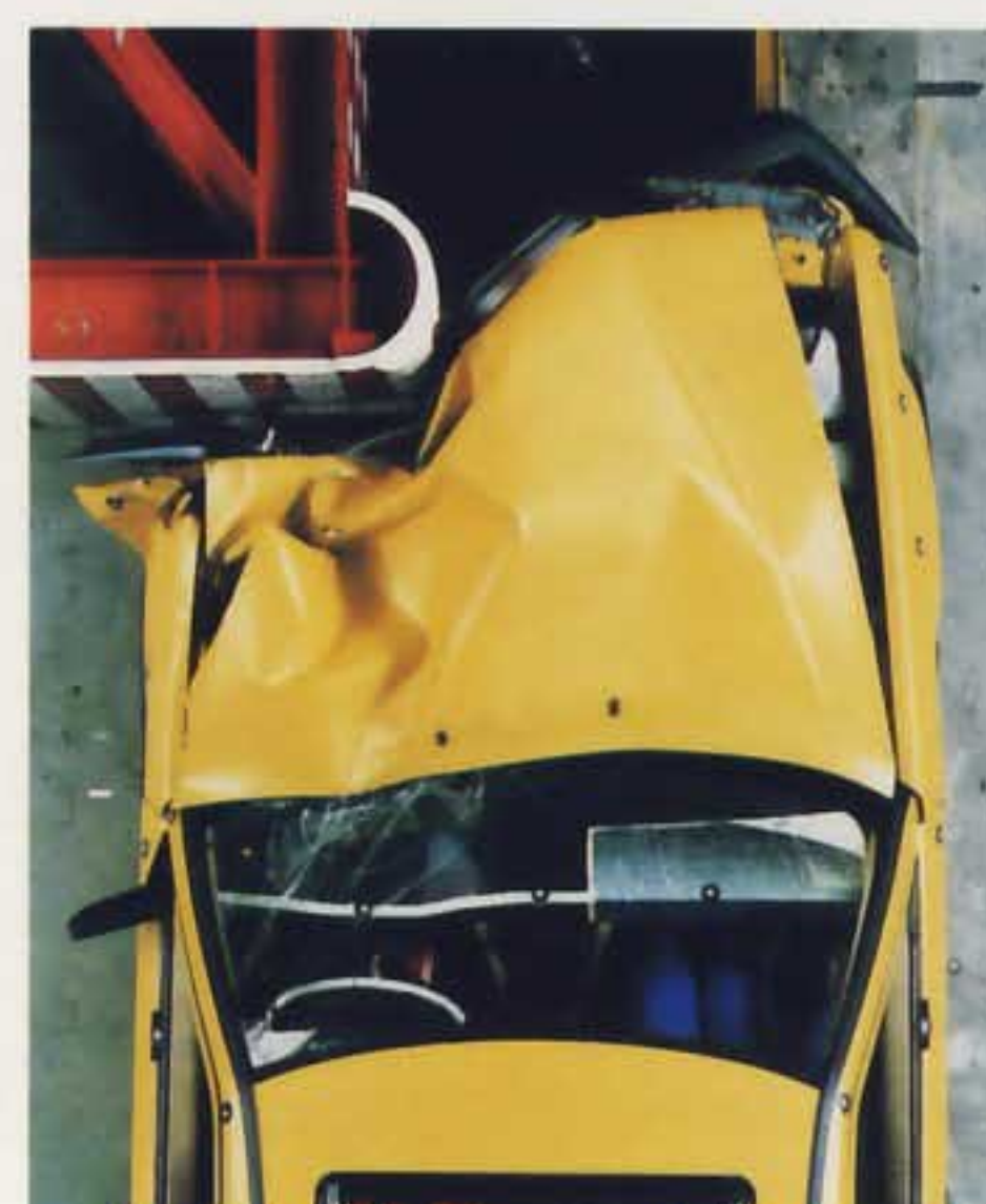
Offset impact testing
