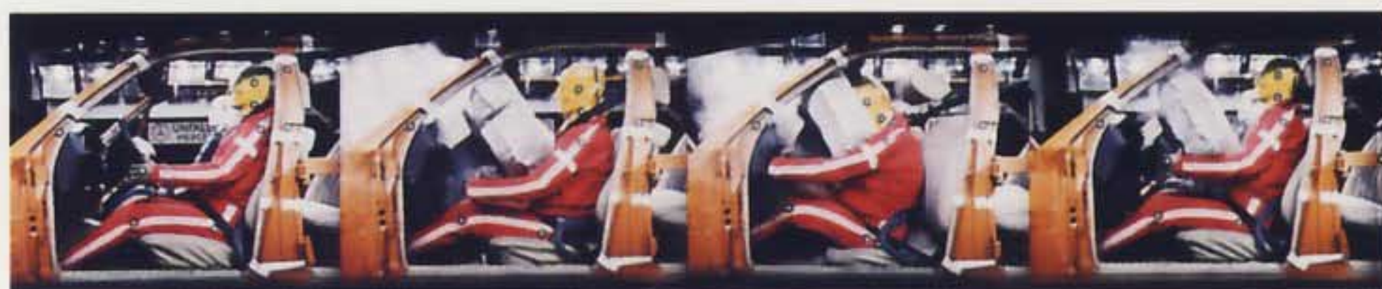
A micro-second review of air bag operation
