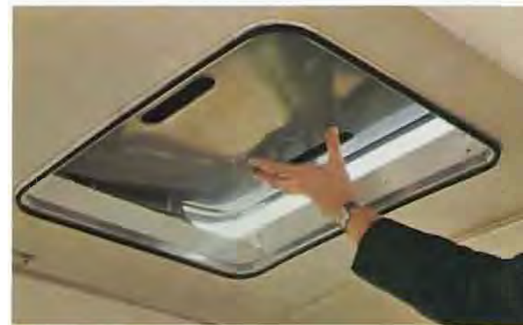
The pop-up roof ventilator, one of nine fresh-air sources.
