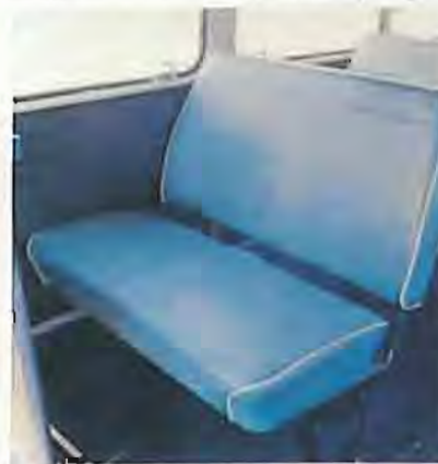
Standard seats for the 13- and 16-passenger versions are constructed with hand-tied coil springs.
