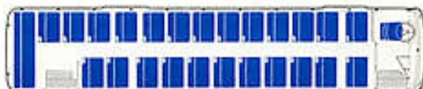
1/108 55 seats, standing room for 51, for commuter service 55 seats, 13 center aisle seats, total weight up to 35,270 lbs (16,000 kg)
