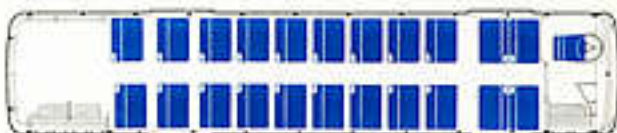
1/98 Basic type, 48 seats, standing room for 50, total weight up to 35,270 lbs (16,000 kg)
